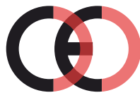
False CE Mark (too close)
